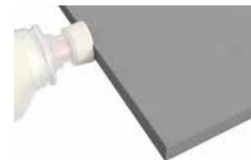
All cut edges (except Cembrit Patina design line boards) must be sealed with Cembrit Edge Sealer to ensure protection of the cut edges. Use the Cembrit Edge Sealer Set with Applicator and Sponge. Avoid getting Edge Sealer liquid on board faces. If this does occur, remove any liquid with a lint-free cloth immediately.
