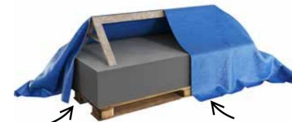
Replace the plastic with a tarpaulin. It is very important that there is ventilation all around the tarpaulin and also on top of the pallet under the tarpaulin. This is done to make sure that condensation is reduced as much as possible.
