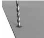
Rivet - Fixing point hole diameter  $\varnothing 10\text{mm}$ . Insert a Cembrit Fixing Sleeve in the hole before the rivet is fixed.
