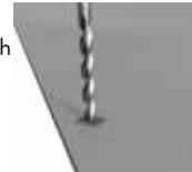
Rivet - Fixing point hole diameter  $\varnothing 10\text{mm}$ . Insert a Cembrit Fixing Sleeve in the hole before the rivet is fixed.
