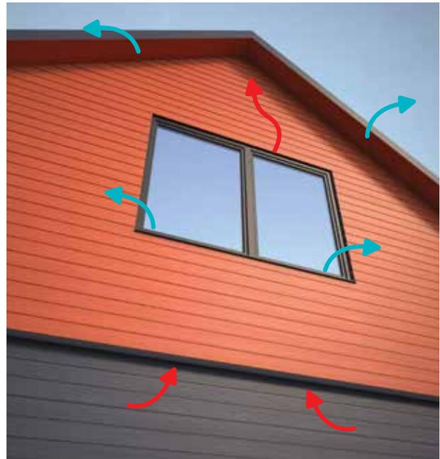
This passage must be a minimum of 10mm in the top and bottom or equal to 100mm per m<sup>2</sup>. If grids or similar are used, the openings must equal 100cm<sup>2</sup> per linear meter.
