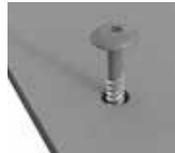
Rivet - Fixing point hole diameter  $\varnothing 9\text{mm}$ . Insert a Cembrit Fixing Sleeve in the hole before the rivet is fixed.
