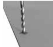
Rivet: pre-drilling in facade board with  $\varnothing 9\text{mm}$  and in steel with  $\varnothing 4.8\text{mm}$
