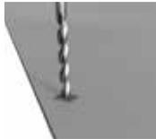
Cembrit Facade Screws should be installed centrally located in pre-drilled holes. The screw must be angled 90 degrees to the facade board. When inserting the Cembrit Facade Screw, please be careful not to overtighten the screw.
