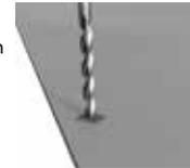
Rivet - Fixing point hole diameter  $\varnothing 9\text{mm}$ . Insert a Cembrit Fixing Sleeve in the hole before the rivet is fixed.
